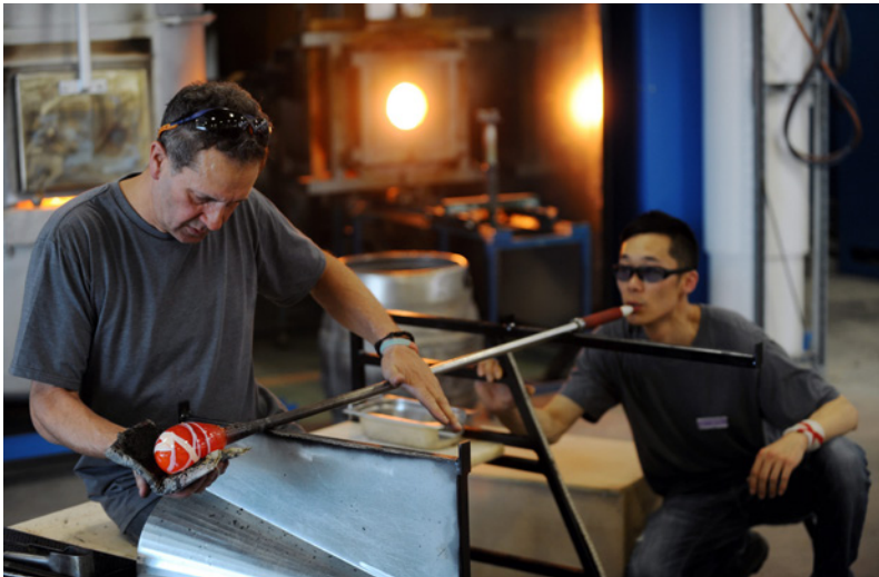
Glass blowers at National Glass Centre work together in teams to handle the hot glass while it is still molten.
