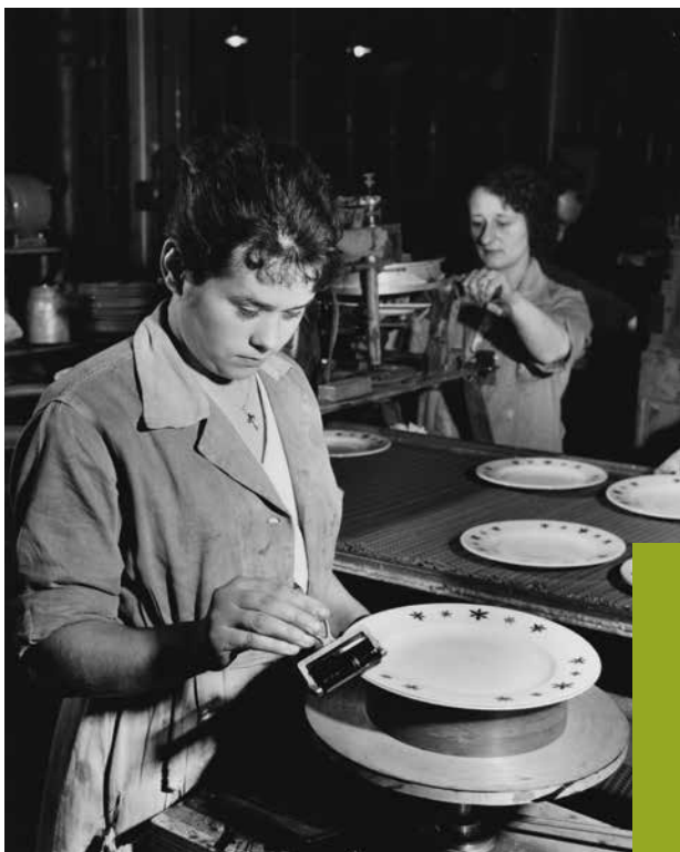
A Pyrex worker concentrating while they apply a gold rim to the edge of the plate.
